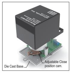
The cover can be removed by loosening the two screws to expose the adjustable close position cam. To adjust the close position from fully closed to about 50% closed, loosen the screw, rotate the cam clockwise and tighten the screw.
